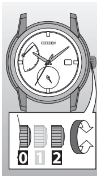
When the watch stops, wind the mainspring manually before setting.
