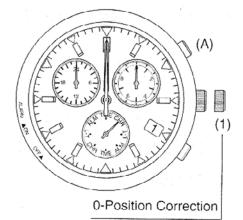
24 hour hand: 24:00 Hour and Minute Hands: 0:00 Second Hand 0:00 seconds Function hand '0' position (12:00 position) Date Wheel 1<sup>st</sup> Perform the "0-position correction" when the hands and date wheel are not at the positions indicated above.
