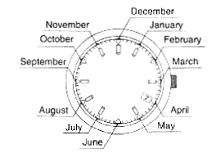
5. Return the crown to the normal position after setting the date. The watch will resume keeping time once the second hand catches up to the current seconds.
