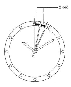
The second hand changes to two-secondinterval movement to indicate insufficient recharging.
