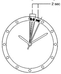
If the watch stops, subsequent exposure to light allows the 'quick start' function to start again, and the second hand moves with a hitch to indicate that the time incorrect.
