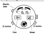
In the same way, to make adjustments while in the calendar mode, press and hold button (B) for more than 2 seconds to select the digit to adjust (will flash), then press button (A) to adjust.
