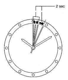
If the watch stops, subsequent exposure to light allows the 'quick start' function to start again, and the second hand moves with a hitch to indicate that the time incorrect.
