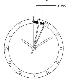
The second hand changes to two-secondinterval movement to indicate insufficient recharging.
