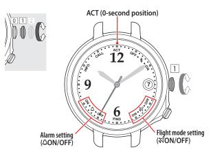
Each time you rotate the crown, the second hand moves as follows: Alarm setting(△ ON/OFF) → ACT → flight mode setting (ズ ON/OFF) → (back to the top).
