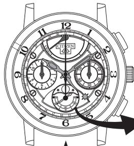
The second hand changes from 1-second interval movement, and the charge indicator hand points at "CHARGE".
