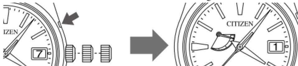
⚠ While holding down the button with a narrow-tipped object, keep your eyes on the tip of the object.
