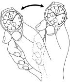
Swing the watch back and forth over a distance of about 20-25 cm (8-10 in.) at the rate of about 2-2.5 strokes per second.
