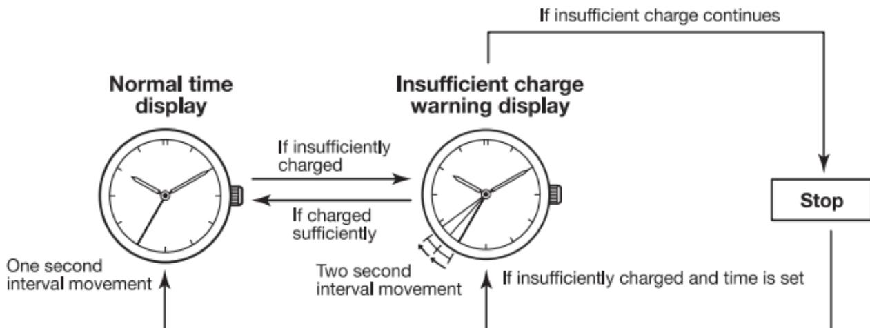
When the watch is exposed to light, the Quick Start Function will begin operating and the second hand will start moving. The correct time can be set once the watch is fully charged.
