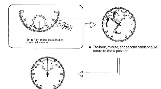
At this time, when each hand is at the position indicated below, the position of the zero setting is correct.
